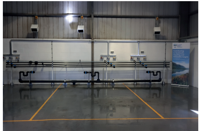
Testing bays at the Bo'ness Development Centre, showing the three different waste water feeds and the pipework to return final effluent to the adjacent treatment works inlet
